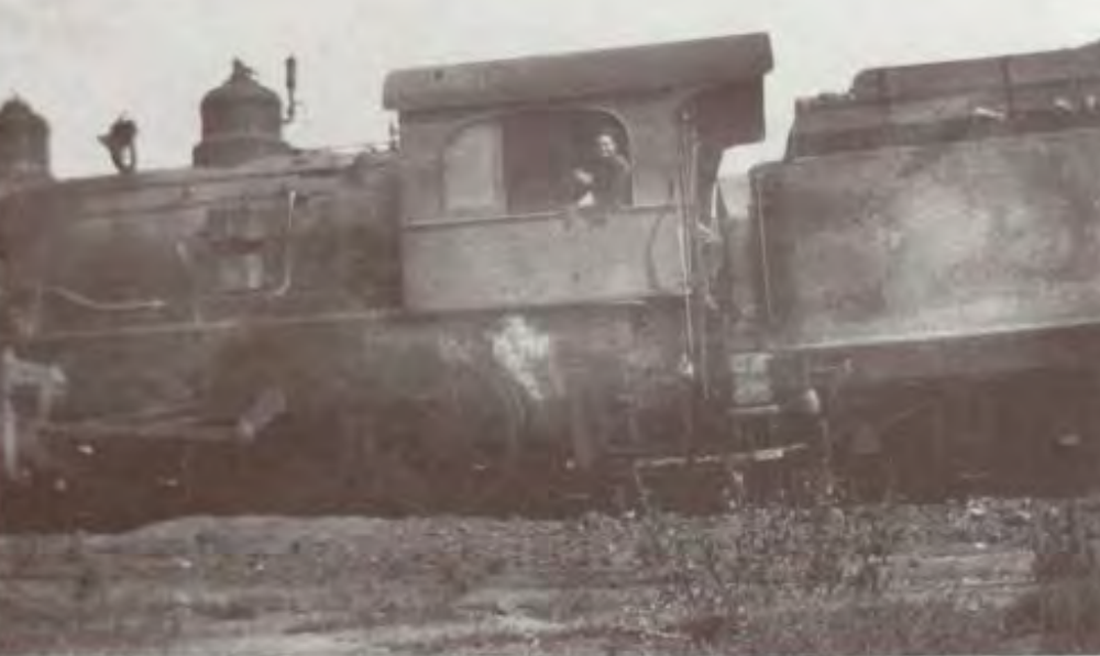
The New Mexico Central had a mixture of second-hand locomotives. This one, built for the El Paso and Northeastern by Baldwin, was acquired in 1919. The curved cab window confirms prior EP&NE ownership. Photograph H. J. Maxwell Collection.
